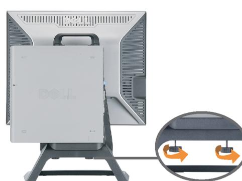
**3 Tighten the screws underneath the stand.**
