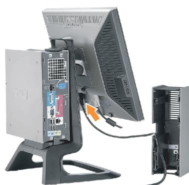
**5 Connect the power cable to the monitor as shown.**
